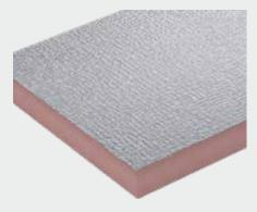
**SUPERCEL® ALUMEN** is a high performance rigid thermoset with resin insulation core with aluminum vapor barrier foil facing covering the upper side and an internal saturated glass tissue facing covering the lower side.
