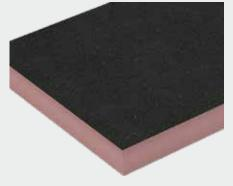
**SUPERCEL® FLAMMA** is a high performance rigid thermoset with a resin insulation core, a mineral added paper based facing covering one side and a graphite based membrane covering the other side. The latter facing should be placed on the side that risks being exposed to flames, guaranteeing both high fire performance and hydro-repellency.
