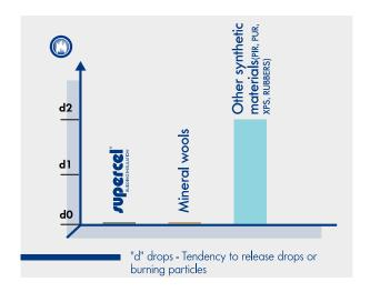
The category s1 guarantees that **SUPERCEL® BUILDING** (together with mineral wools, i.e. non-synthetic materials) is a product with extremely **low smoke emissions** and toxic gas emissions such as carbon dioxide and carbon monoxide. This distinguishes it from all other synthetic materials, such as XPS, PIR and PUR, and from vegetable fibres (*see table*).
